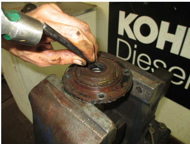
9. Once it is far enough out, the race can be hit from the other side with a punch to get it the rest of the way out. (switch side-to-side, so it comes out relatively straight)
