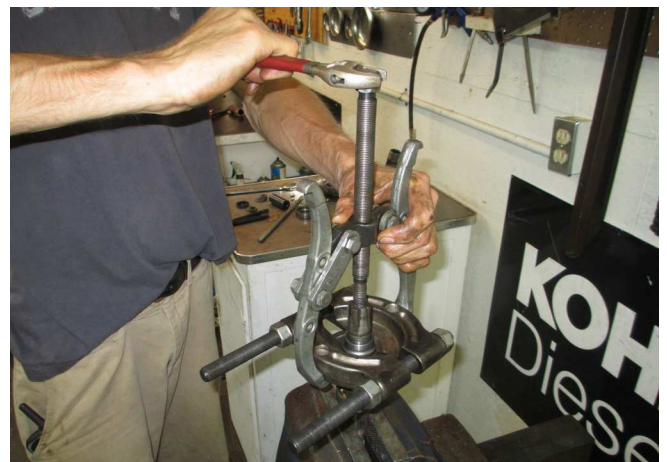
10. If the bearing (8 & 9) did come apart, the inner race remains on the shaft. It can be removed using the tools pictured, or by carefully grinding through the inner race on one side, so it will “open up” and fall off the shaft easily. (BE CAREFUL not to damage the seal-surface of the shaft, or the shaft is ruined!) NOTE: a good machine-shop can get these races out too...
