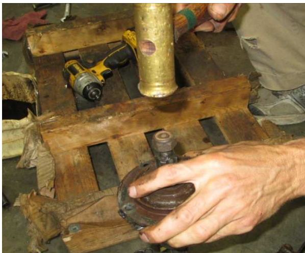
7. The shaft can be driven out of the cover with a brass hammer, while holding the cover, or positioning the cover over an open vise, etc. to support it. Again, BE SURE TO HAVE A NUT ON THE THREADS!
