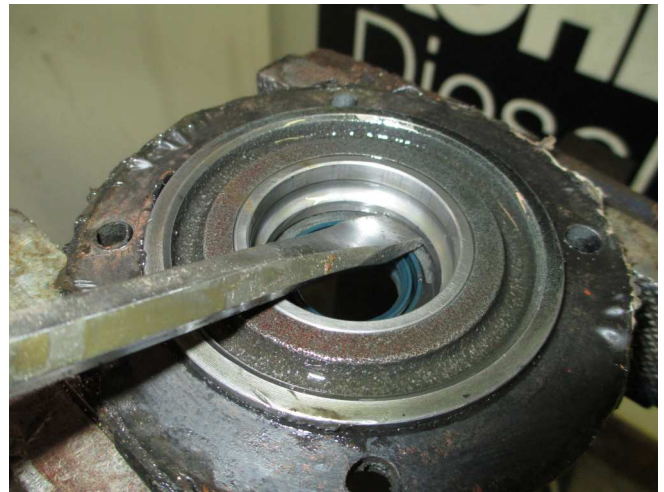
8. On older units, it is not uncommon for the cover-side bearing to come apart, leaving the outer race of the bearing in the cover. If this happens, it can be “walked out” with chisels (increasing size as it moves out...wedge under one side, then the other).
