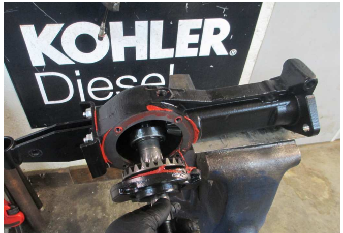
6. Note the use of silicone gasket maker. Silicone should be reapplied when reassembled. NOTE: May have to use one or more gaskets (part # 580.43407) to set the gear lash properly (BCS does not list this part on the new part listings, but we have them!!).
